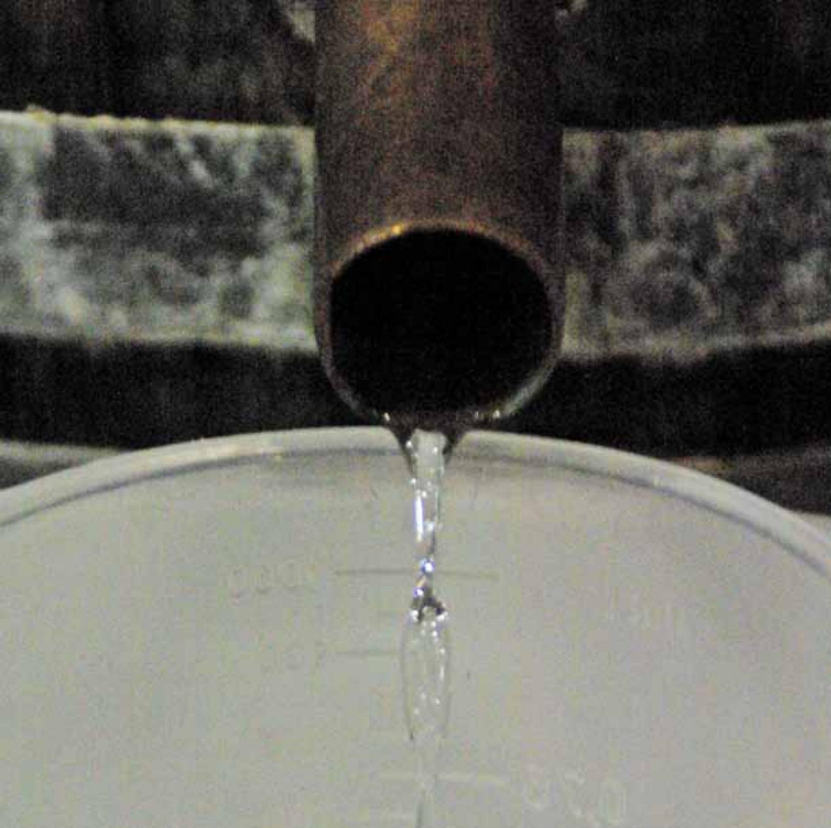
Windsor Run Cellars operates a still in Hamptonville, North Carolina. Several wines are fortified with brandy. The brandy is made from the grapes grown on the property. The liquid shown in the photo is the heads. This will not be used in fortifying wines. After the heads, the tails are what a winemaker is looking to use.
